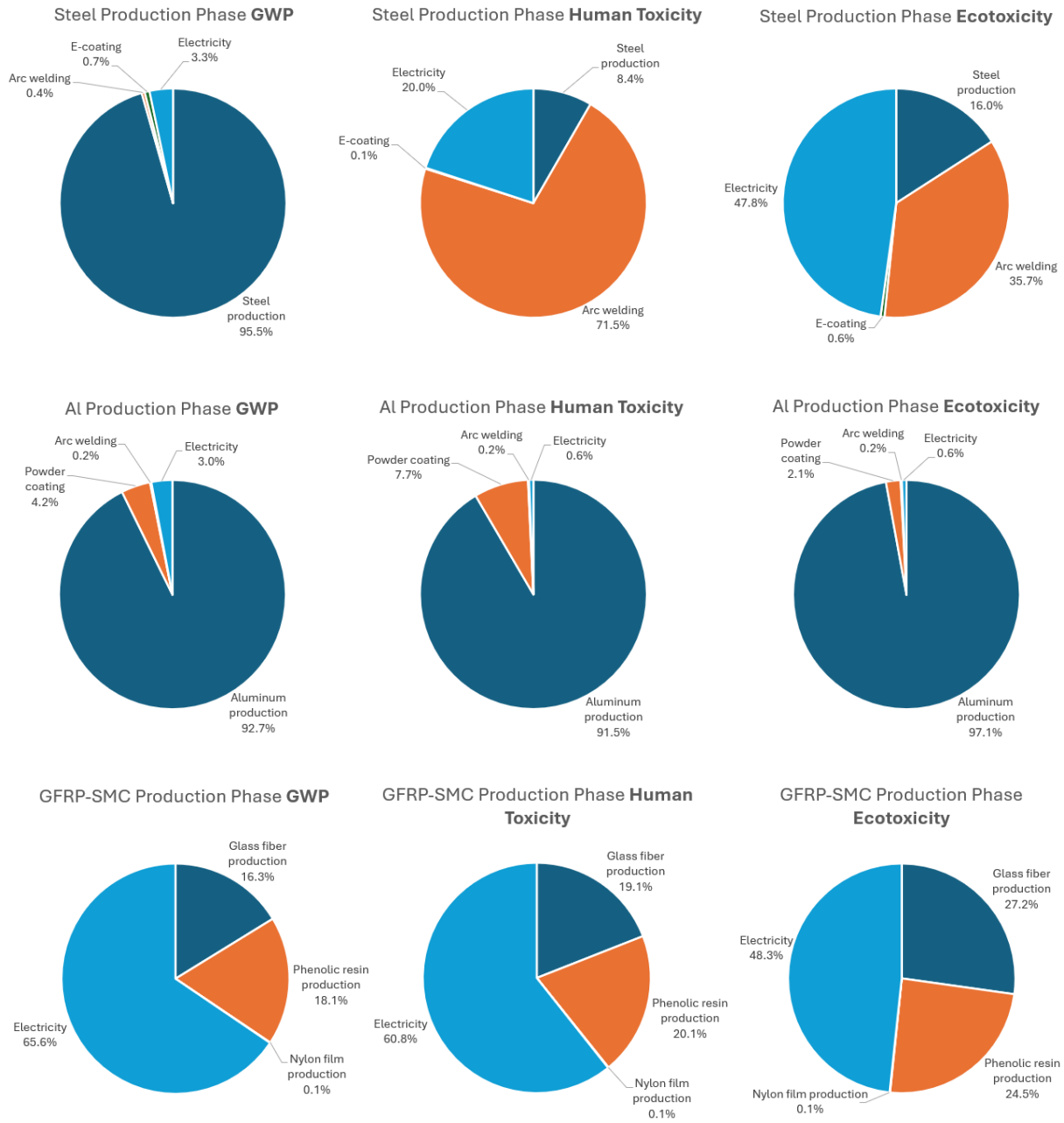
Figure 12. Breakdown of battery box production phase impact by material and process.
